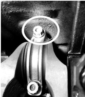
Make sure there is 1.0mm to 1.5mm of clearance between the connecting rod and the cylinder block.
