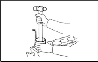
① Before assembling, apply oil to the cylinder wall, piston outer surface, and the connecting rod bearing.
