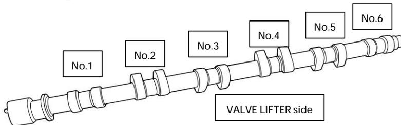
Be careful not to over tighten the cam cap bolts on lobes #1, #2, #4 and #6.
