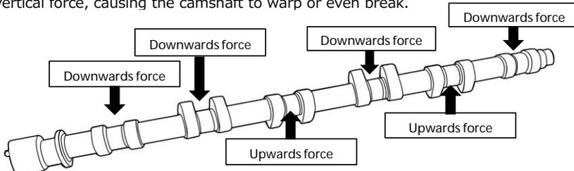
When installing the camshafts, ensure that you tighten down the bolts slowly and evenly so that the camshaft sits level in the cylinder head.
